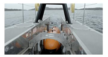
The **SEA-KIT X FST** includes a multibeam echo sounder, station holding and underwater vehicle launch and recovery packages to deliver versatile ocean survey capability. When equipped with a swarm of AUV/UUVs, large areas of the ocean can be surveyed by the vessel and its assets fully autonomously. The extended endurance and robustness of the X Class allows for surveys many miles from port or mother ship.
