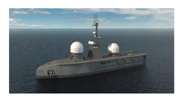
The **SEA-KIT XL FST** includes a multibeam echo sounder, station holding and underwater vehicle launch and recovery packages to deliver versatile ocean survey capability. When equipped with a swarm of AUV/UUVs, large areas of the ocean can be surveyed by the vessel and its assets fully autonomously. The extended endurance and robustness of the XL Class allows for surveys many miles from port or mother ship.
