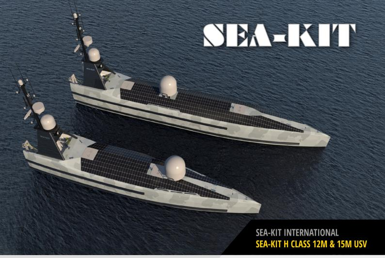
The SEA-KIT H-Class USV's highly configurable design, with a retractable gondola and dual sensor deployment options, is based on a wealth of operational data and feedback collected from the company's proven and established X-Class USVs.
