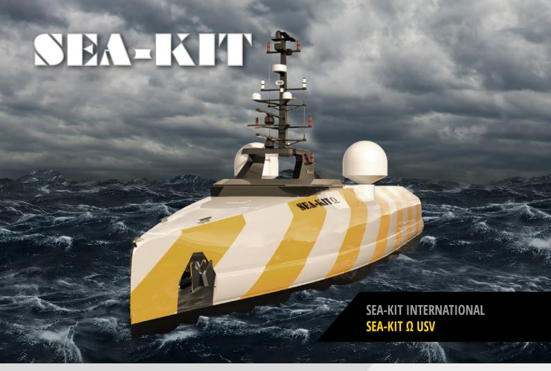
The SEA-KIT Omega Uncrewed Surface Vessel (USV) is designed for extended endurance, fully uncrewed maritime operations. With a large payload capacity and the capability to autonomously launch, recover and control subsea vehicles, including ROVs and AUV/UUVs, SEA-KIT Omega meets the demands of current and future offshore operations above and below the water.
