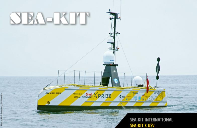
SEA-KIT X is a remotely controlled, versatile and configurable mother-ship platform that can launch and recover remote vehicles such as large AUV/UUVs or ROVs, enabling missions including deep-water bathymetry, offshore and subsea asset inspection and hydrographic survey with reduced risk to personnel, significantly decreased costs and lower environmental impact.
